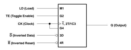
logic diagram, each D/T flip-flop (positive logic)
